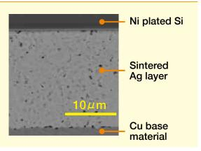
Silver nanoparticles promote fusion between silver powders to strengthen thermal and electronic moving pathways.
