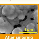
SEM observation result of cross-section of joining part
