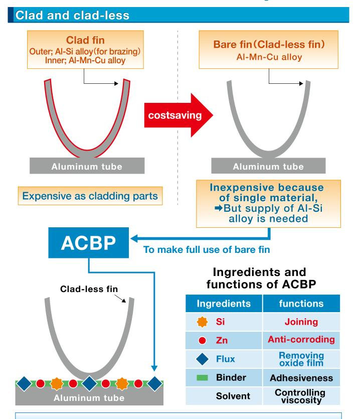
Make it possible to provide not only joining but also anti-corroding
